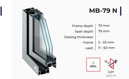
$^*$  U\_w for the MB-79N SI system with reference window dimensions of 1230x1480 mm, with glazing U\_g=0.5 W/(m²K), with warm spacer SSP Ultimate.
