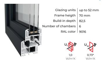
\* U\_w value for U  $_{\rm g}$  =0.5 with warm spacer SSP Ultimate, values are given for reference window dimensions of 1230x1480 mm.
