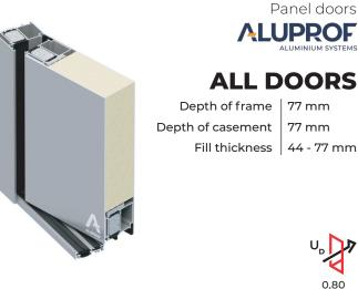
\* - Ud for door MB-86N SI+ with casement dimensions 1400x3000 mm, with glass Ug=0,5 W/(m2K), with warm swisspacer advance
